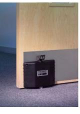
Fire doors should only be held open by a device that will automatically release if there's a fire. Some doors may be fitted with magnetic devices linked to the fire alarm that would release automatically. These are very expensive to retrofit. Alternatively, there are standalone, battery-operated devices known as Dorgards that should release when the fire alarm sounds.
